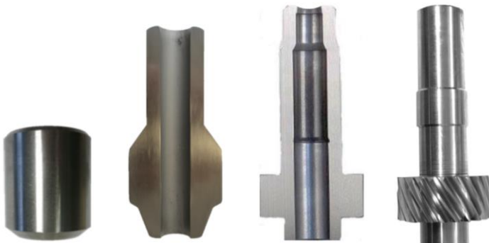
Image: The shortened demonstration process chain depicts all steps for the production of geared hollow shafts by means of forming. Source: © Fraunhofer IWU.
